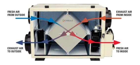
Features of CASALICA plate type heat exchanger:  $\star$  No wear & tear because there is no moving parts  $\star$  Side and corner sealing avoids transfer of odors, contamination or humidity  $\star$  High efficiencies due to special plate design  $\star$  Different plate distances (spacing) are available  $\star$  Horizontal or vertical installation is possible  $\star$  Low investment cost  $\star$  No electrical connections  $\star$  Light-weight, compact design, easy to install
